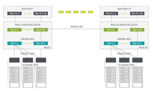
Figure 1: Typical cloud data center deployment for the QFX5700
