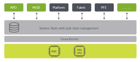
Figure 2: Cloud/Carrier-Class Junos OS Evolved Network Operating System
