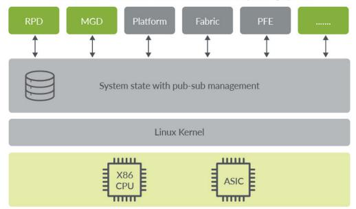
Figure 4: Cloud/Carrier-Class Junos OS Evolved Network Operating System
