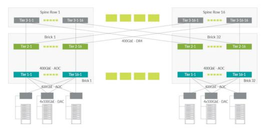
Figure 1: Typical cloud data center deployment for the QFX5220-32CD
